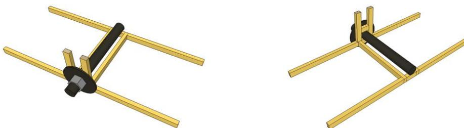
Figure 3. **Recommended strengthening near the mass**
